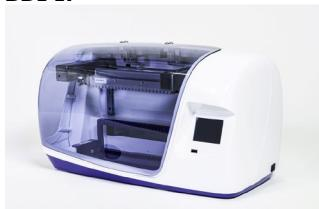
The BDI I is an instrument that performs the various steps of incubation and washing of D-tek's immunodot strips, from the deposit of the sample to the final colour development. The maximum capacity is of 24 strips which are incubated simultaneously. Each strip is associated with a cartridge containing the various reagents making it possible to carry out the test. The BlueDiver Instrument has a barcode reader which controls the correct association between a strip and its cartridge.
