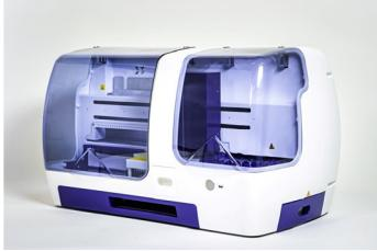
The BlueDiver Instrument II is an instrument that performs the various steps of samples pipetting, incubation, washing, drying and reading of D-tek's immunodot strips, from the deposit of the sample tube to the final reading of the strips.
