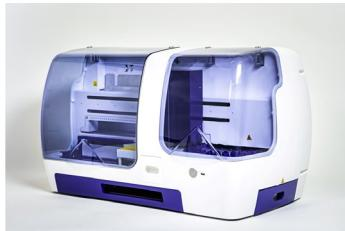
The BlueScan and Dr Dot Software are intended for reading test results of D-tek immunodot strips. The Dr Dot Software and BlueScan scanner must be used in combination.
